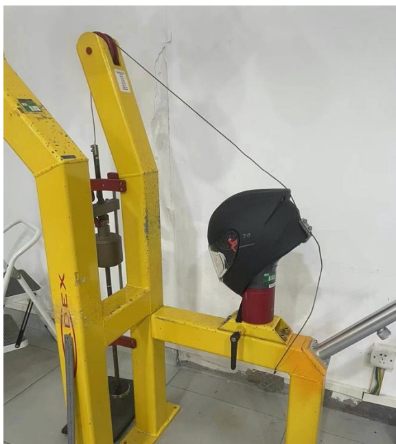
Retention detaching test
